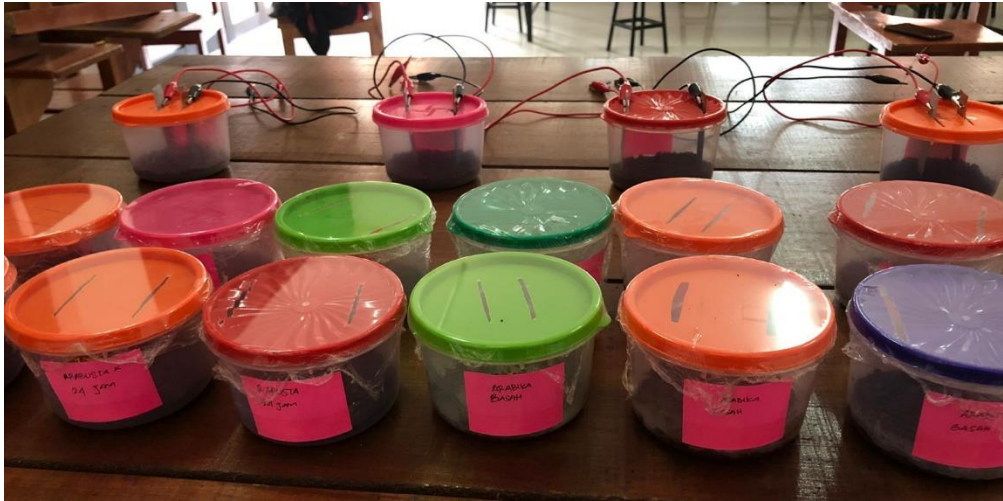
Figure 2. Electrical characteristic and stability test of coffee grounds biobattery
