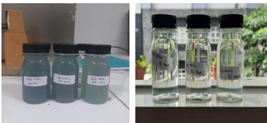
Fig.2 Leachate of nickel slag extraction (a) before destruction (b) after destruction
