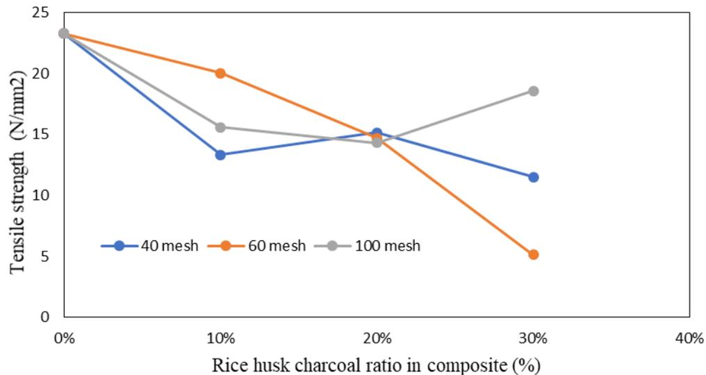
**Fig.2.** The relationship between tensile strength and particle size of rice husk charcoal for 0, 10, 20, and 30 % ratio charcoal in composite
