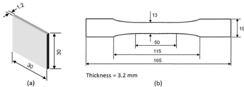
Fig.1. Specimens with standard size ASTM D-638-4
