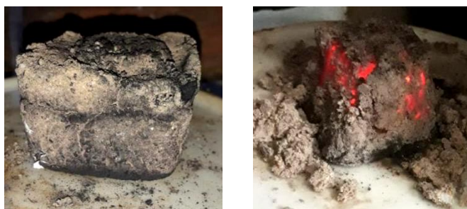
Fig.7. Observation result during combustion of bio-briquettes
