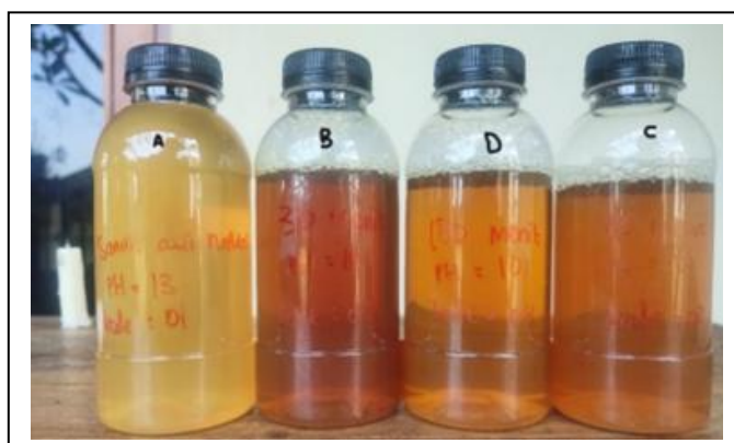
Fig. 2 The difference in color before and after adsorption, a) original batik liquid waste, b) after adsorption for 30 minutes, c) after adsorption for 90 minutes, d) after adsorption for 180 minutes.
